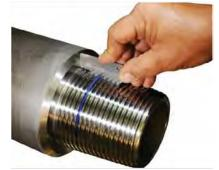
LPP on a Pin with blue line marking proper thread
